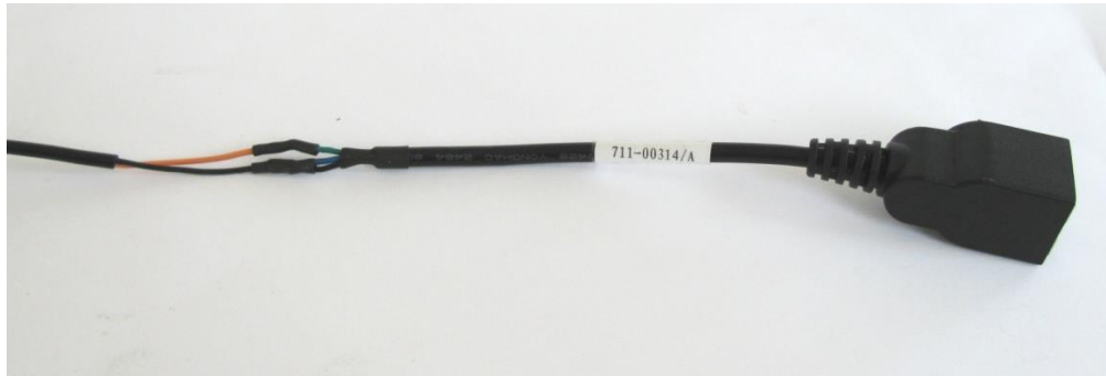
Figure 2: Cello Harness prepared for 1-wire Temperature Sensor installation
